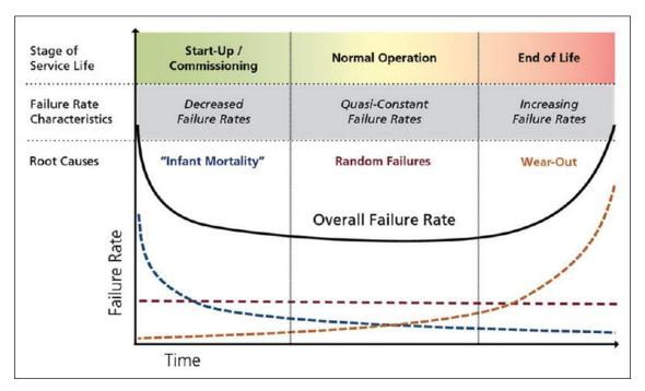
The 'Bathtub Curve' timeline of failure Hazard function (black solid line) incorporates rates of early failure (blue dotted line) with end of life wear-out failure (yellow dotted line), and continuous, unchanging random failure rates (red dotted line)
